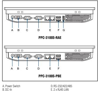
D. RS-232/422/485 E. 2 x RJ45 LAN F. 1 x USB 2.0, 1 x USB 3.0 G. USB 2.0
